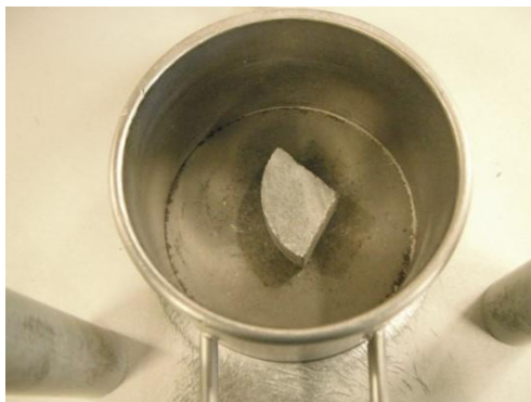
Figure 8. Cut-Core Fragment Produced with the Diamond Saw
