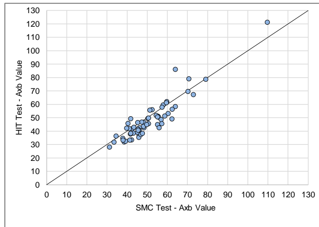
Figure 4 – Comparison of SMC Axb Values and Corresponding HIT Axb Proxy Estimates (62 drill core samples)
