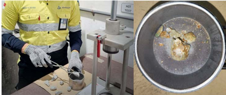
Figure 4—Image of HIT device at Batu Hijau and close-up of broken rock in cup
