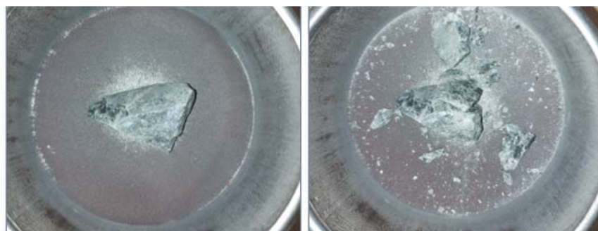
Figure 10—Example of 22.4 x 19 mm fragment before and after breakage in the HIT
