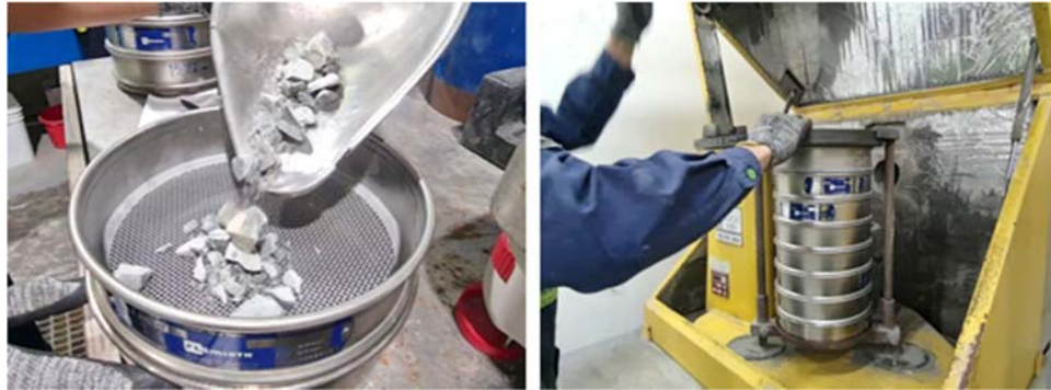
Figure 11—Sieving of HIT breakage products post breakage test
