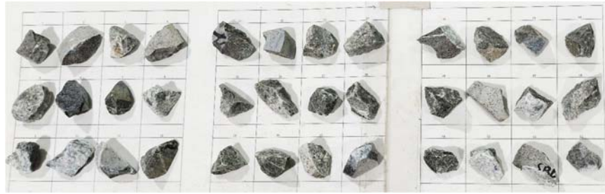
Figure 8—Crushed fragments from P7AC and P8 core samples ready for AxB measurement using HIT
