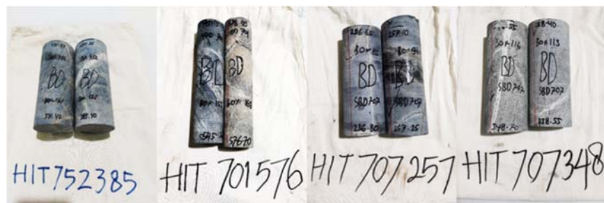
Figure 7—Batu Hijau P7AC and P8 core samples selected for Axb measurement using HIT
