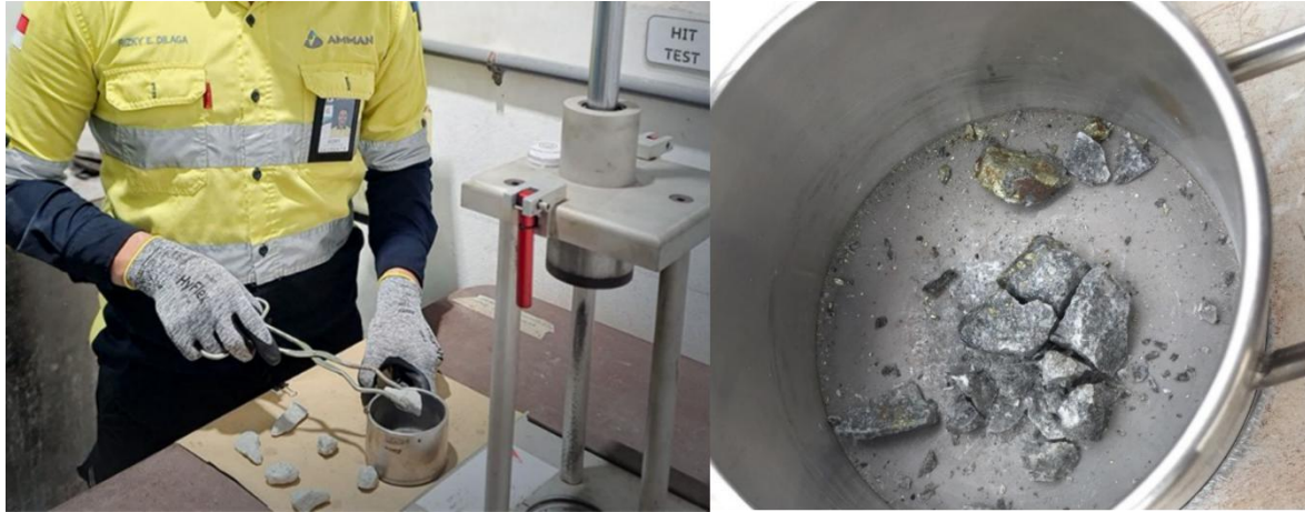
Figure 1: Image of HIT device at Batu Hijau and close-up of broken rock in a cup
