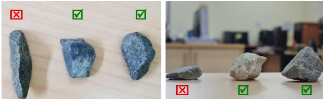
Figure 3: Example of rejected and accepted 22.4x19 mm fragments
