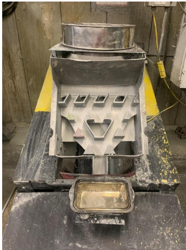
Figure 4: Image of Gibraltar screening station to remove 16x13.2 mm fragments for HIT Axb test
