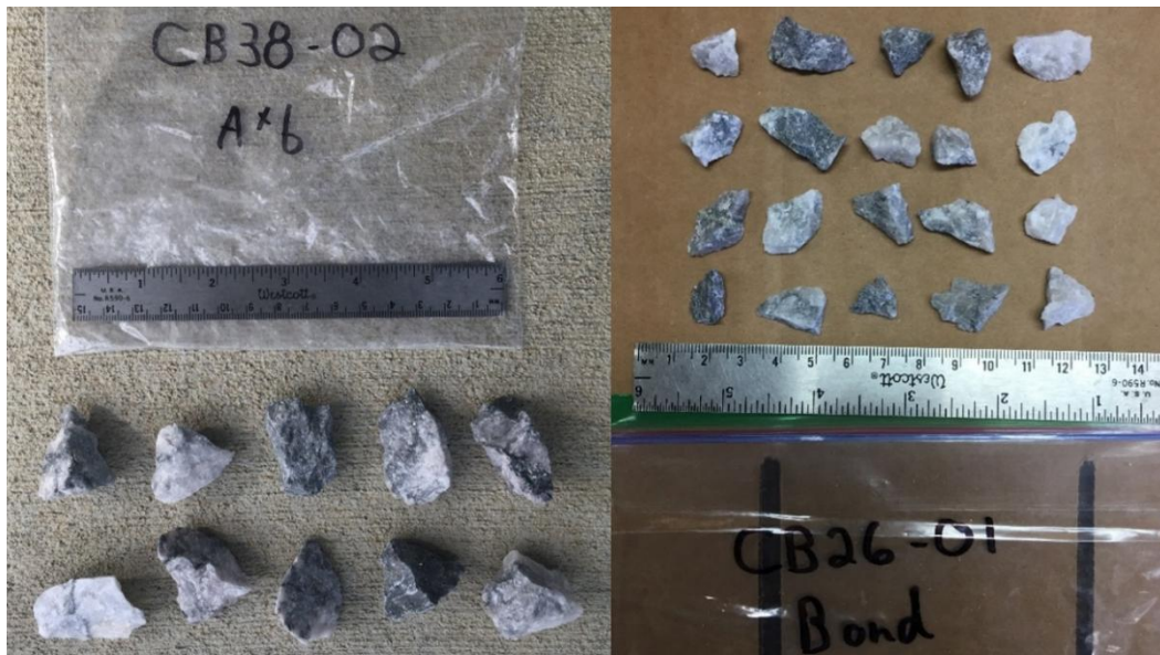
Figure 2: Image of Hecla 22.4x19mm fragments for HIT Axb test and 11.2x9.5 mm fragments for HIT Bond BWi HIT test
